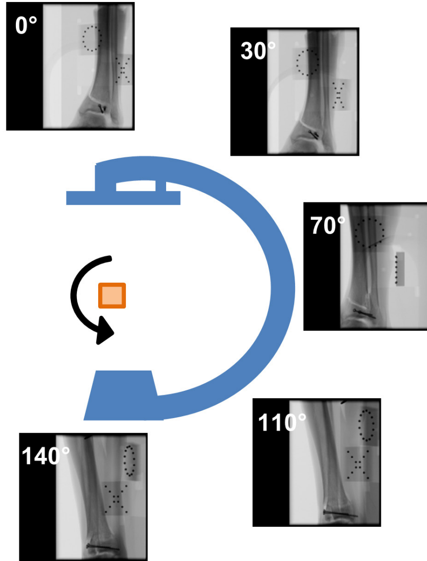
Figure 3.22: Evaluation of calibration methodology was performed by taking 16 images spaced at 10 degree rotations about the gantry.
